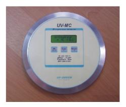
The UV-MC Microprocessor Integrator is a self-contained, high quality UV measuring instrument. It is designed to measure, record and display peak UV intensity, UV dosage and temperature in the UV curing process.
