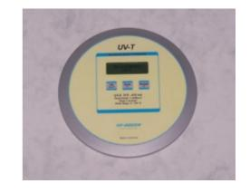
The UV-T Microprocessor Integrator is a self-contained, high quality UV measuring instrument. It is designed to measure, record and display peak UV intensity, UV dosage and temperature in the UV curing process.
