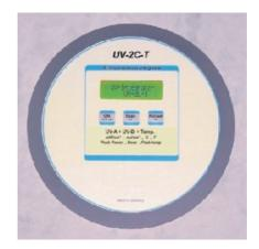
The UV-2C-T Microprocessor Integrator is an economical, self-contained, high quality UV measuring instrument. It is designed to measure, record and display peak UV intensity and UV dosage in the UV curing process.
