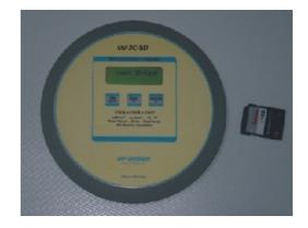
The UV-3C SD Microprocessor Integrator is a self-contained, high quality UV measuring instrument. It is designed to measure, record and display peak UV intensity and UV dosage in the UV curing process.
