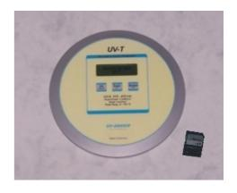
The UV-T SD Microprocessor Integrator is a self-contained, high quality UV measuring instrument. It is designed to measure, record and display peak UV intensity, UV dosage and temperature in the UV curing process.
