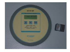
The UV-3C-T SD Microprocessor Integrator is a self-contained, high quality UV measuring instrument. It is designed to measure, record and display peak UV intensity, UV dosage and temperature in the UV curing process.
