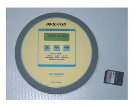
The UV-2C-T SD Microprocessor Integrator is an economical, self-contained, high quality UV measuring instrument. It is designed to measure, record and display peak UV intensity, UV dosage and temperature in the UV curing process.
