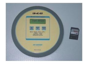
The UV-4C SD Microprocessor Integrator is a self-contained, high quality UV measuring instrument. It is designed to measure, record and display peak UV intensity, UV dosage in the UV curing process.
