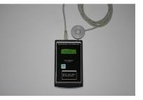
All measurements are expressed in mW/cm<sup>2</sup> in order to compare light sources or to check uniformity of the light emission.
