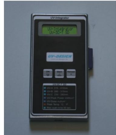
The **UV-2C Microlog SD with SD Memory card** is a self-contained, high quality UV measuring instrument. It is designed to measure, record and display peak UV intensity, UV dosage (and temperature \* option) in the UV curing process.
