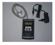
The UV-Probe Integrator is a self-contained, high quality UV measuring instrument. It is designed to measure and display UV energy in mW/cm<sup>2</sup>. An additional function is the scan of the peak value of UV-intensity in mW/cm<sup>2</sup> and to measure the UV dose in mJ/cm<sup>2</sup> within a pre-set period of 30/60 seconds.
