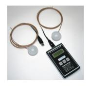
The UV-Probe Integrator Multi is a self-contained, high quality UV measuring instrument. It is designed to measure and display UV intensity in mW/cm<sup>2</sup>. An additional function is the scan of the peak value of UV-intensity in mW/cm<sup>2</sup> and to measure the UV dose in mJ/cm<sup>2</sup> within a pre-set period of 30/60 seconds.
