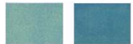
After continued UV exposure, the Labels take on a deeper shade of green, eventually reaching their maximum exposure color, solid blue.
