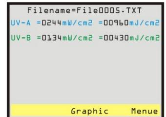
With these two different UV-bands many of the measuring requirements of UV curing applications can be covered. Due to its two different UV sensors and the integrated microprocessor the **UV-1200 Colour RE Radiometer + Dosimeter** can measure, record and display the peak of the UV-intensity ( $mW/cm^2$ ) for each UV-band individually plus the peak of total UV energy.
