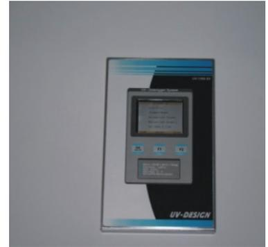
The **UV-1200 Colour RE Radiometer + Dosimeter** is a self-contained, high quality UV measuring instrument. It is designed to measure and record UV intensity, UV dosage and temperature in the UV curing process. Measuring results are indicated both, graphically and numerically on a big colour display.
