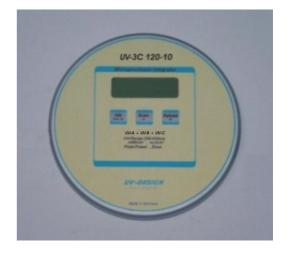
The UV-3C Integrator 120-10 is a self-contained, high quality UV measuring instrument. It is designed to measure and display peak UV intensity, UV dosage and temperature in the UV curing process. Thank to its special dimensions it is particularly suitable for the CD and DVD production.
