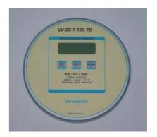
The UV-2C-T Integrator 120-10 is a self-contained, high quality UV measuring instrument. It is specially designed to measure and display peak UV intensity and UV dosage in the UV curing process of CD and DVD production.
