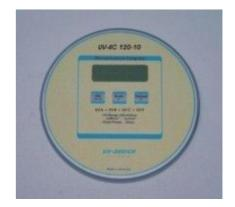
The UV-4C Integrator 120-10 is a self-contained, high quality UV measuring instrument. It is designed to measure and display peak UV intensity, UV dosage and temperature in the UV curing process. Thank to its special dimensions it is particularly suitable for the CD and DVD production.
