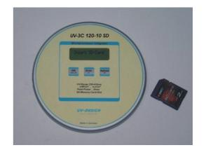
The UV-3C Integrator 120-10 SD is a self-contained, high quality UV measuring instrument. It is designed to measure, record and display peak UV intensity, UV dosage and temperature in the UV curing process. Thank to its special dimensions it is particularly suitable for the CD and DVD production.
