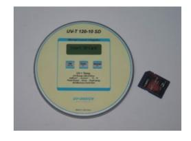
The UV-T Integrator 120-10 SD is a self-contained, high quality UV measuring instrument. It is designed to measure, record and display peak UV intensity, UV dosage and temperature in the UV curing process. Thank to its special dimensions it is particularly suitable for the CD and DVD production
