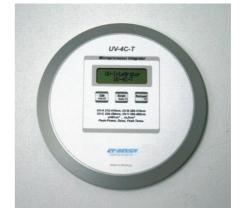
The UV-4C-T Microprocessor Integrator is a self-contained, high quality UV measuring instrument. It is designed to measure, record and display peak UV intensity and UV dosage in the UV curing process.
