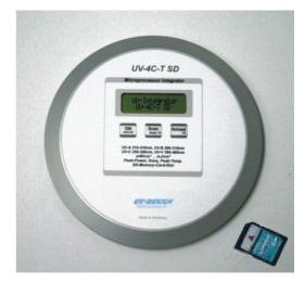
The **UV-4C-T SD Microprocessor Integrator** is a self-contained, high quality UV measuring instrument. It is designed to measure, record and display peak UV intensity, UV dosage in the UV curing process.
