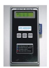
The **UV-4C-T Microlog SD** is a self-contained, high quality UV measuring instrument. It is designed to measure, record and display peak UV intensity, UV dosage and temperature in the UV curing process. It is equipped withfour different UV sensors and one temperature sensor for the individual measuring of
