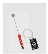
The UV Rigid Probe Integrator is a self-contained, high quality UV measuring instrument. It is designed to measure and display UV energy in mW/cm<sup>2</sup>. An additional function is the scan of the peak value of UV-intensity in mW/cm<sup>2</sup> and to measure the UV dose in mJ/cm<sup>2</sup> within a pre-set period of 30/60 seconds.
