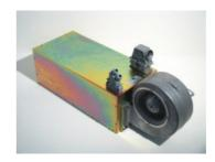
The EVG UV 62-70 AC is a fully electronic, adjustable AC ballast unit for UV-lamps from approx. 6 kW - 12 kW nominal power and specially designed for industrial use. It is specially tuned to operate with mercury discharge UV-lamps of  $15 - 70 \text{ cm} (6^{\circ} - 27^{\circ})$  arc length. Dark phases during the zero axis known from standard, sinus shaped power supplies are eliminated by operating the lamps with a square-wave current.
