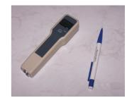
The UV-Spot Curing intensity Meter 5-10 is a high quality electro-optic UV measuring instrument. It is self-contained, battery-operated, portable, light-weight and easy to handle. It is specially designed to measure and display peak UV intensity emitted by UV spot curing
